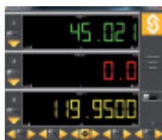
Multi channels screen with tolerances displayed in colour
