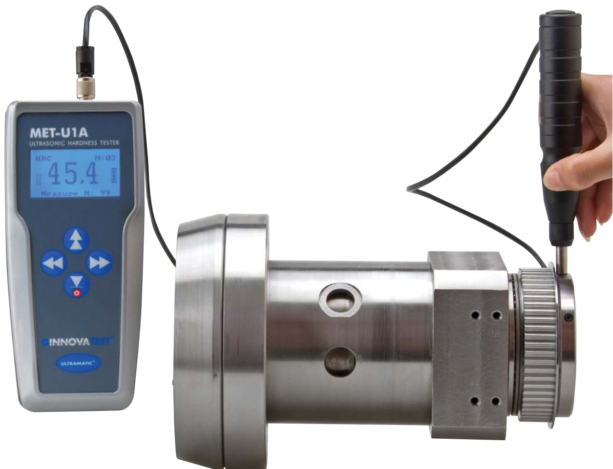
MET-U1A ULTRASONIC HARDNESS TESTER, 15N TESTFORCE
