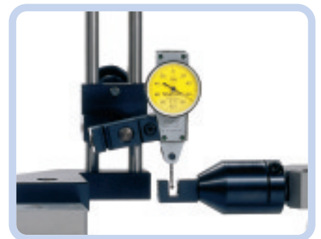
Checking of test indicator
