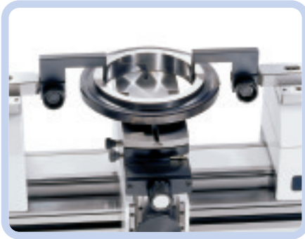
Checking of ring gauges
