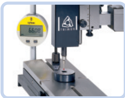
Checking of ring gauges
