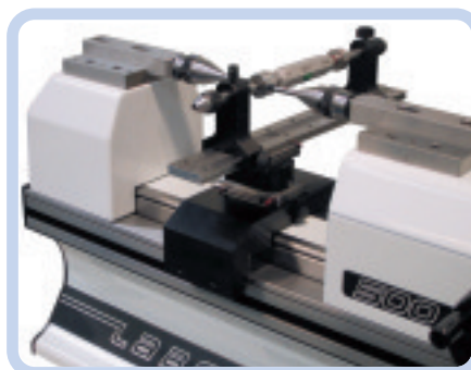
Checking of thread plug gauges using LABC - 15
