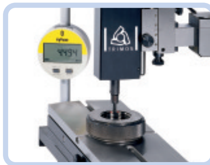
Checking of thread ring gauges
