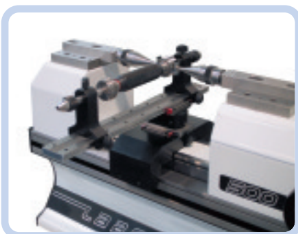
Checking of plug gauges using LABC - 15
