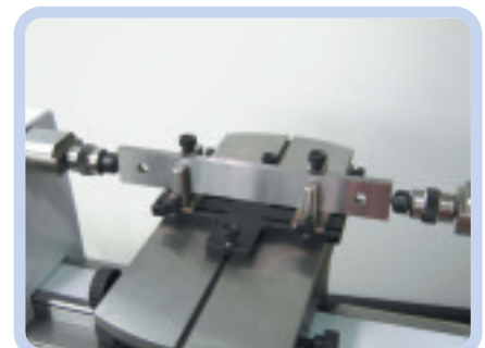
Checking of gauge blocks up to 250mm (250 to 1000mm)
