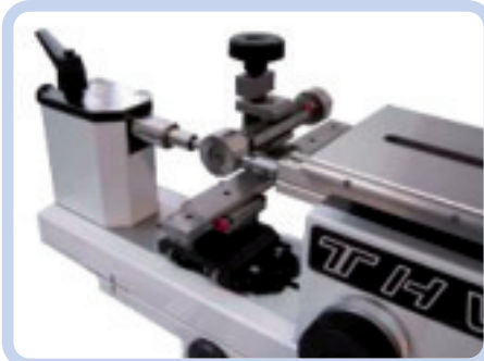
4) Checking of plain and threaded plug gauges using the floating table
