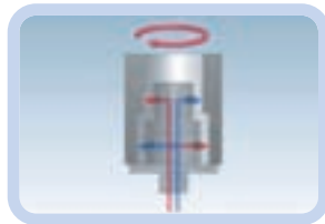
Concentricity of 2 Inside Diameters
